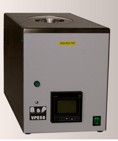
ried out by a PID microprocessor controller. This control technique results in high level of reproducibility and repeatability of the test results. The limits quoted in DIN 51581, ASTM D5800/a and CEC L-40-A-93 can be easily observed with large safety margins.
